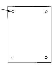
4. Hold one of the acrylic sign panels at the desired location on the wall and make sure it's level. Pencil in the hole locations onto the wall. Drill pilot holes for the screws and if your wall is hollow insert the wall anchors.
